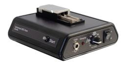
The Splice-On Connector (SOC) Curing Oven for 3.0mm and 900um is powered by a Li-Ion battery and provides maximum portability and flexibility for field installation. Adjustable heat cycles allow this curing oven to be used with connectors for 3.0mm or 900um fiber cables.
