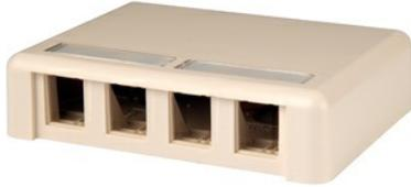
Ortronics 4 port high density jack (HDJ) Surface Mount Outlet Box accept 4 jack modules and provides snap-on covers and snap-in label fields. 4.75" x 3.6" x 1.15". Box is supplied with screws and double-sided adhesive tape for mounting onto almost any surface.
