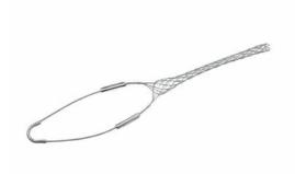
FC150U: Standard Duty, Closed Mesh, Single-Eye Grip, Cable Diameter 1.50 - 1.74 inches, Bale Length 12-in, Mesh Length 18-in, Break Strength 1680 lbs.
