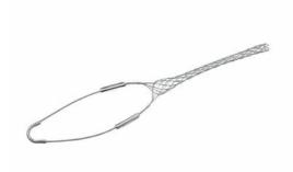
FC175U: Standard Duty, Closed Mesh, Single-Eye Grip, Cable Diameter 1.75 - 1.99 inches, Bale Length 14-in, Mesh Length 20-in, Break Strength 2640 lbs.
