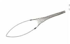
FC200U: Standard Duty, Closed Mesh, Single-Eye Grip, Cable Diameter 2.00 - 2.49 inches, Bale Length 16-in, Mesh Length 22-in, Break Strength 3760 lbs.
