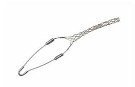
FCSD40: Service Drop, Closed Mesh, Single Eye, Cable Diameter 0.41 - 0.56 inches, Bale Length 6-in, Mesh Length 5-in, Break Strength 500 lbs.
