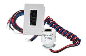
The LMFC-xRJ provides fixture connectivity to the DLM local network via a single- or dual-port RJ45 wiring whip connector. The dual-port is best for daisy chaining multiple fixtures together. Each DLM local network can support up to 64 loads.
