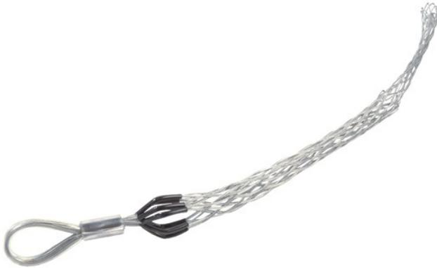
Multi-Weave, Rotating Eye. Cable Diameter - 3.000-3.490-inch, Mesh Length - 54-inch, Eye Diameter - 1 7/8-inch, Break Strength - 48,000 lbs, Aluminum.
