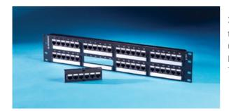
24- and 48-port TechChoice® patch panels are available in the traditional multi-port panel format with 6-port modules for Cat6 and Cat5e. Patch panel kits are also available to support individual keystone jacks. This is a Category 5e patch panel, 48-port, universal T568A/B wiring, six-port modular, 2 rack units.
