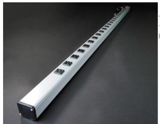
Twenty-four outlets, rugged gray aluminum housing, 15A, lighted switch, 15' (4.6m) 14/3 SJT black cord with NEMA5-15 plug. Length 72'' (1.8m). Receptacle center-to-center 2 1/2'' (64mm). Snap-on, slide-off mounting.
